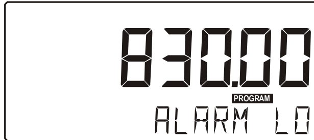
Fig. 4: Example of display information during programming minimum flowrate.
