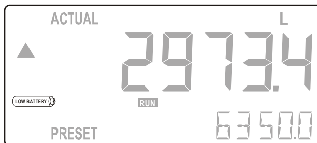
Fig. 6: Example of low-battery alarm.
